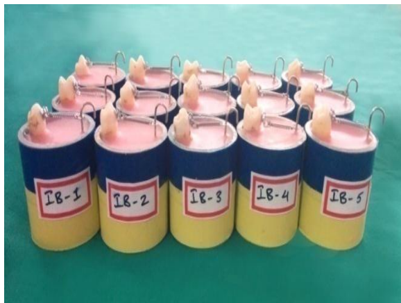
Fig 1. Example of a bonded bracket with the coil applying force.
