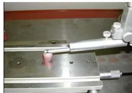
Figure. 5. The sample during Profilometer testing.
