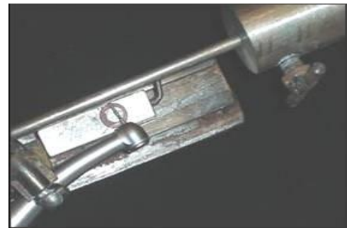
Figure.4. Specially designed device for burs treatment.
