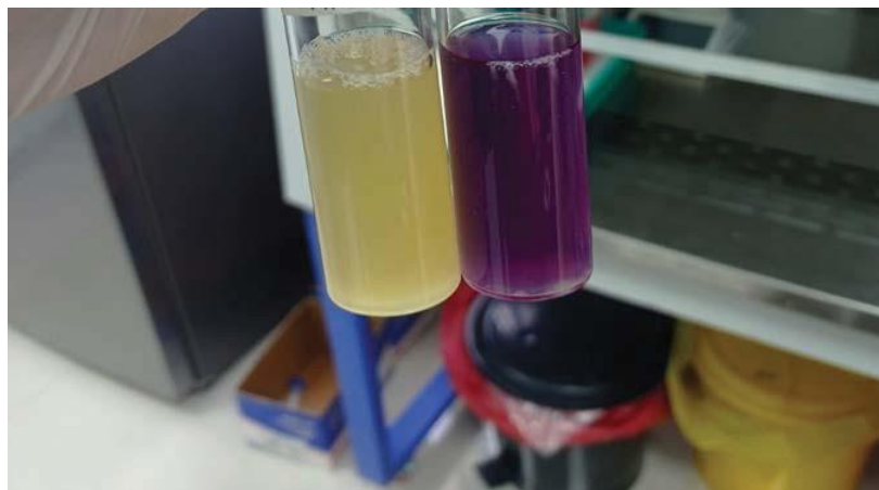
Multiple Tube Fermentation Technique for presumptive Coliform Count
