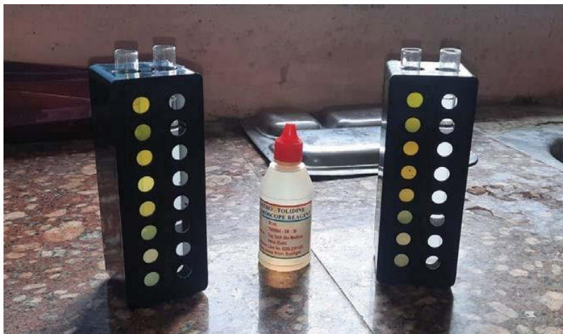
Chloroscope & Ortho-Tolidine Reagent for Assessment of Chlorine level.
