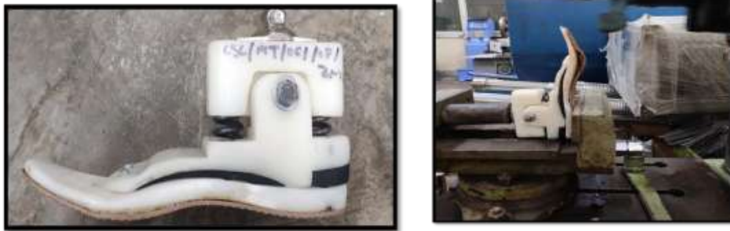
Fig. 6 (a) & (b) mechanical cyclic testing procedure of MPF
