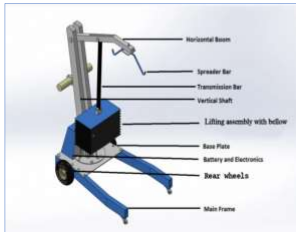
Figure 2. Parts of PLH
