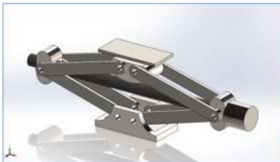
Figure 10. CAD Drawing of Screw Jack
