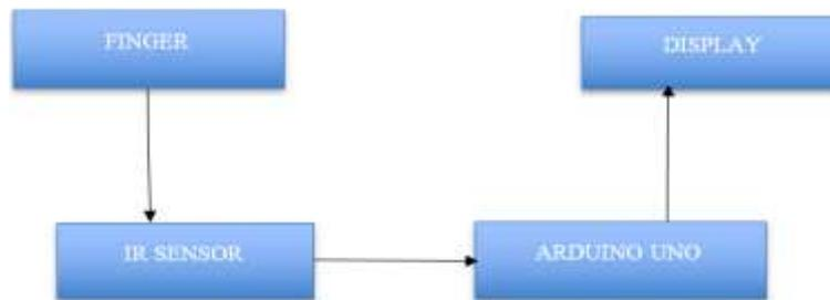
Figure. 02. Block Diagram of the Device
