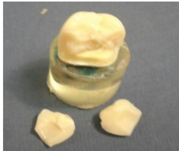
Fig (8): Fracture mode of a representative sample of group IV (Resin Nano Ceramic Lava Ultimate endocrown) leaving the tooth intact (restorable, favorable failure).
