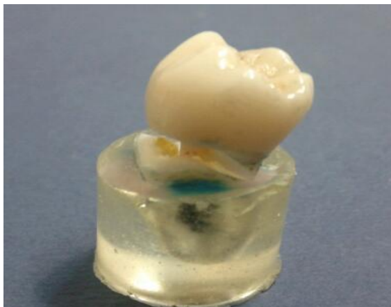
Fig (5): Fracture mode of a representative sample of group I (post and core supported Prettau Zirconia crown) showing root involvement (unrestorable, unfavorable failure).
