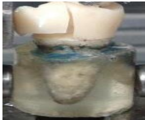
Fig (7): Fracture mode of a representative sample of group III (post and core supported Resin Nano Ceramic Lava Ultimate crown) leaving the tooth intact (restorable, favorable failure).
