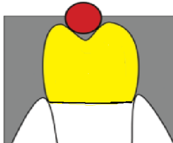
Fig (3): Schematic diagram showing the relationship between the loading element and the tested crown. The loading element is presented by red color, the tested crown is presented by the yellow color while the abutment tooth is presented by the white color.
