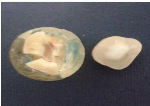
Fig (6): Fracture mode of a representative sample of group II (Prettau Zirconia endocrown) showing root involvement (unrestorable, unfavorable failure).
