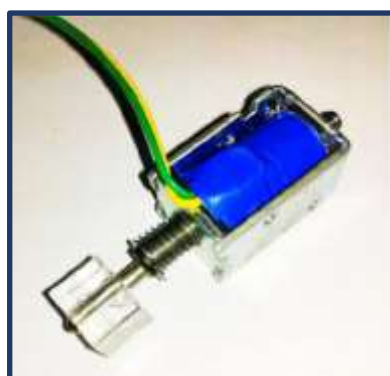
Fig.5: Solenoid used in indigenously developed knee joint with pin attachment and an acrylic block
