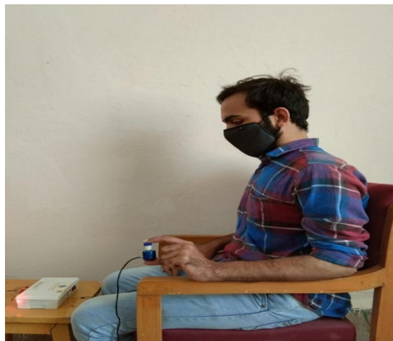
Image 3: Measurement of pinch grip using SVPT device
