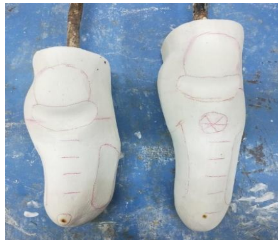
Fig.3 Modified mold with markings
