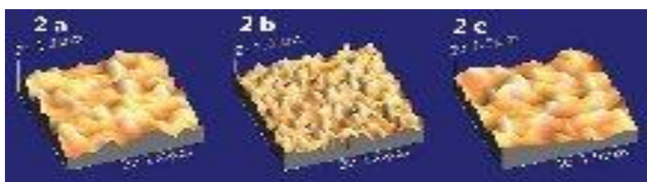
Fig.2: 3D image of the surface profile of the yz ceramic samples after different surface treatments; a. air borne particle abrasion, b. VM9 glaze coating with hydrofluoric acid etching, c. e.max glaze coating with hydrofluoric acid etching. (Magnification x50)
