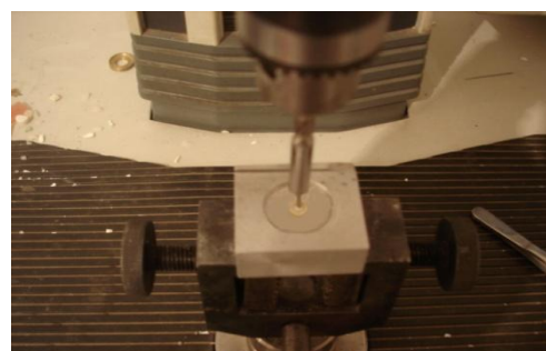
Figure (4): Specimen and attachments used for shear bond strength test.
