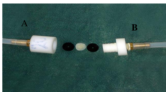
Figure (3): Opened split Teflon chamber device with a pair of rubber "O" rings and a dentin disc. A: female part, B: male part.
