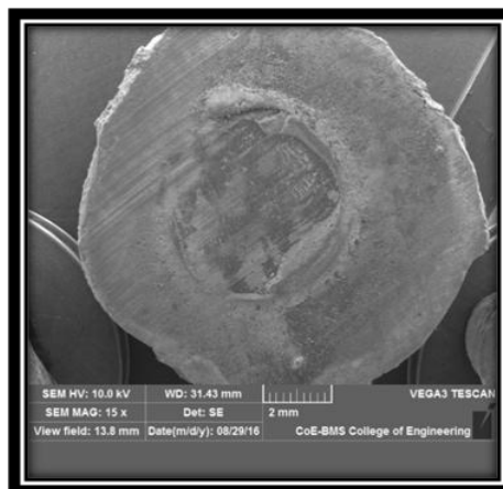
Figure 10(B): Fractured Sites of Core X Flow Core Material and Dentin Interface Showing Adhesive Failure with No Residual Core Material on Dentin Surface
